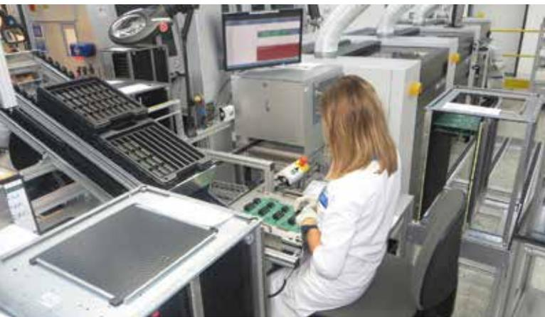
product is positioned, a cavity plate, which covers the soldering bath and the soldering head in order to guarantee a perfect nitrogen atmosphere, is lowered and exposes the soldering head accordingly. Then the entire soldering transport segment is placed on the soldering pre-position; the last 2 mm up to the soldering head are approached slowly, and the soldering process begins.
